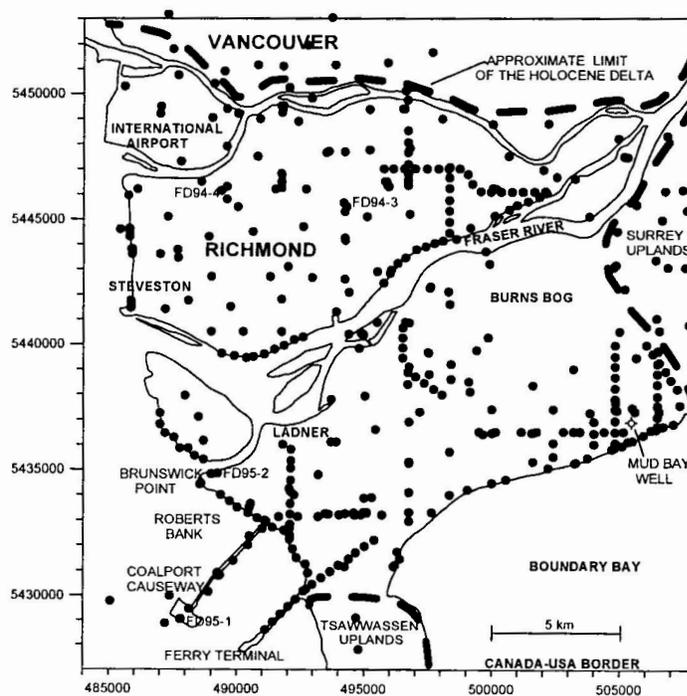
Figure 1. Location of shear wave seismic data sites in the Fraser River delta.
