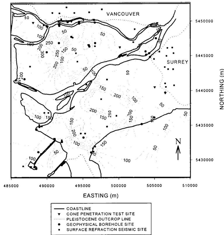
Figure 3. Computer-generated map of estimated depth below surface to the Holocene-Pleistocene shear wave velocity boundary based on available data.
