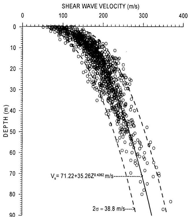
*Figure 2. Compiled shear wave velocities vs depth for Holocene deltaic sediments, Fraser River delta. Every fifth point is plotted for clarity.*
