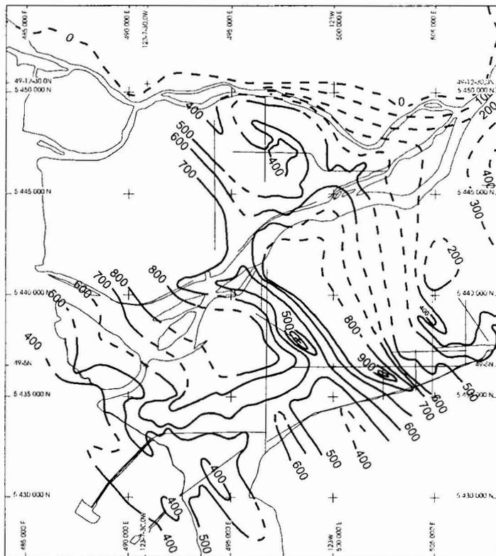
Figure 5. Depth below surface to Tertiary bedrock after Britton et al. (1995), based on seismic reflection measurements.
